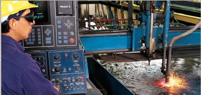
Engineering data files are fed directly into Valmont's CNC controlled plasma burning equipment, creating precisely cut steel components.
