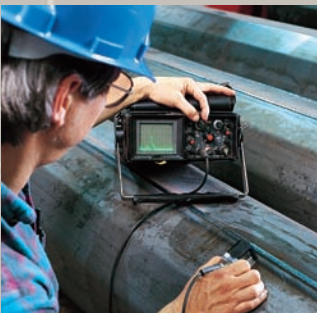
Full penetration welds are always inspected and verified ultrasonically. The component does not progress to the next phase of fabrication until it passes completely.
