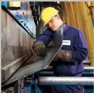
Our 2,000-Ton pressbrake is among the most reliable and powerful in the industry. Limitless combinations of length, diameter, thickness and taper are possible during the forming process.
